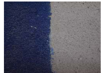
Decomposition of the Blue ink stain, after exposure to sunlight for 5 hours
