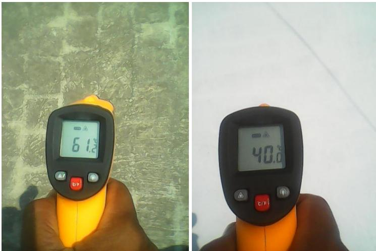
**Lots of customers at Chennai have used Surfapore thermodry mixed with an acrylic emulsion paint for coating the terrace to save energy and reduce heat inside the building. There is a difference of more than 20° C on the surface before and after coating. Surfapore thermodry is a thermal insulation coating which not only reflects more than 93% of IR rays but also cuts the thermal conductivity by 4 times.**
